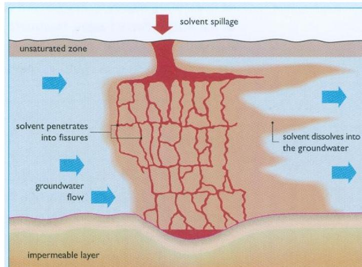
Figure 12. Soil and fractured aquifer pollution by chlorinated solvents spillage. They are denser than water, non-miscible phase liquids (DNPL) that sink slowly through the whole unsaturated zone thickness and cumulate in the aquifer bottom; the plume and main body contaminates groundwater in contact with them due to the slight solubility (Lawrence and O'Dochertaigh, 1998).
