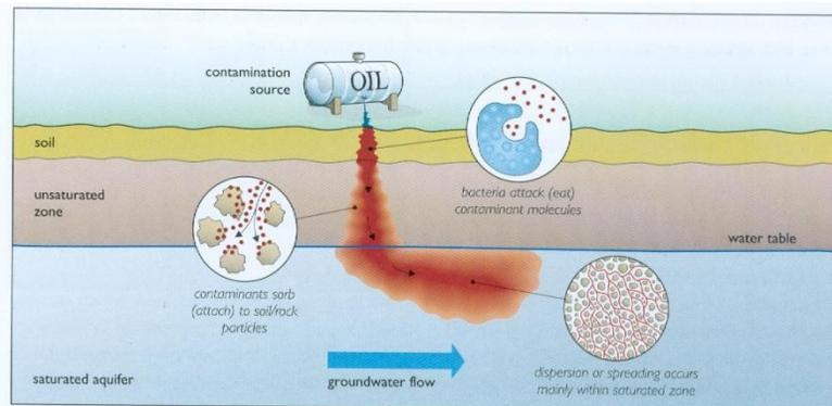
Figure 11. Soil and aquifer pollution by oil tank spills and leakages. Mineral oil is a lighter than water, non-miscible phase liquid (LNPL) that floats on the water table; it is slightly soluble in water and disperses according to water-table fluctuations and groundwater flow (Lawrence and O'Dochertaigh, 1998). Under favourable circumstances, natural processes may help in reducing contamination through degradation, sorption and dispersion.
